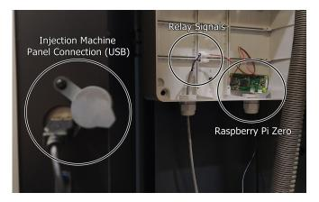
Fig. 2. Real system connected to the injection machine.
