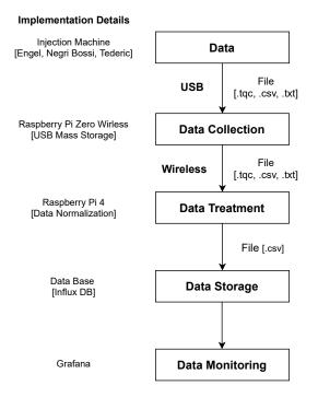
Fig. 1. System Architecture
