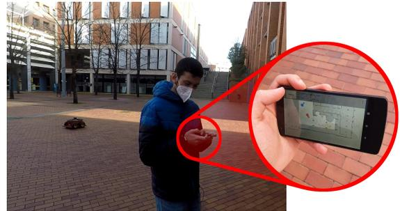
Fig. 1. Participant using our interface to communicate with the robot: It is not necessary to maintain visual contact with the robot at any time.
