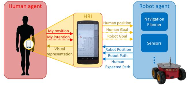
Fig. 2. **Information flow considered in our proposal.** Smartphone acts as an HRI interface converting graphic information understandable by the human into messages understandable by the robot and vice versa.
