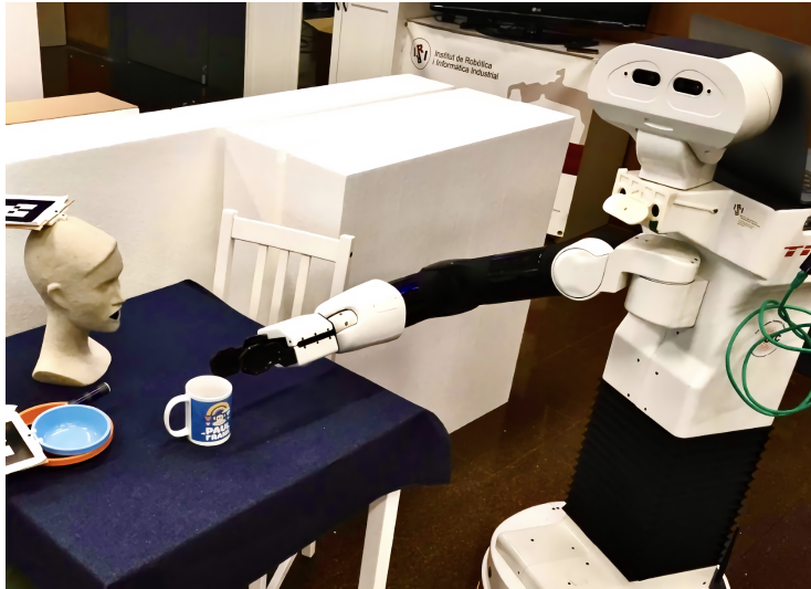
Figure 1: TIAGo robotic platform developed by PAL Robotics performing a manipulation task.
