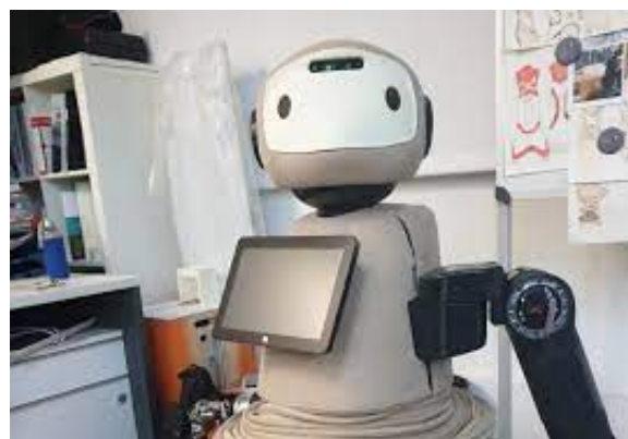
Figure 1. IVO Robot. New design of a humanoid robot for citizen assistance.
