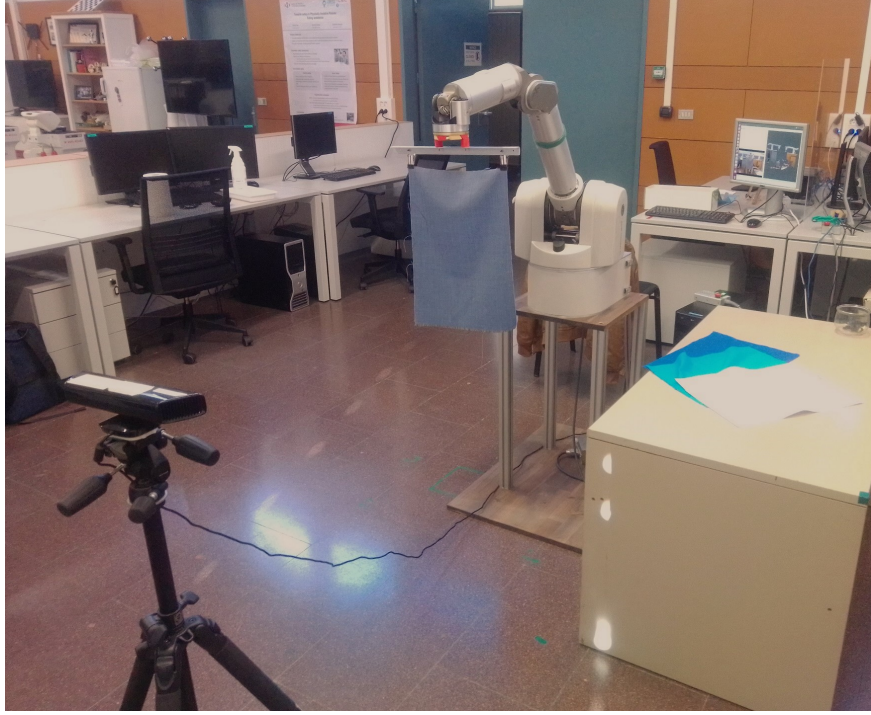
Figure 3: Experimental setup for the recording of real world data. On the left, the depth camera. On the right, the robotic arm with an affixed hanger.
