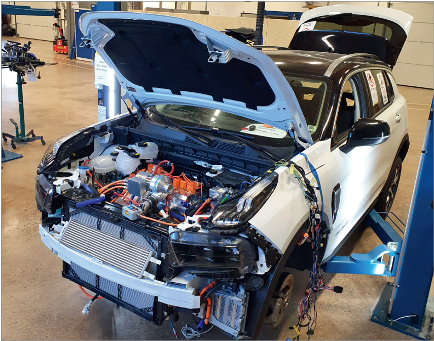
Figure 12: Fuel cell system implemented in the vehicle powertrain, Source: China Euro Vehicle Technology AB.
