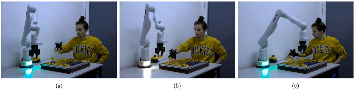
**Fig. 8.** Plan adaptation to unforeseen events. In the shown sequence, (a) the human and the robot move towards the same compartment; (b) then the human fills the compartment; (c) the robot adapts its plan and moves to another free compartment.
