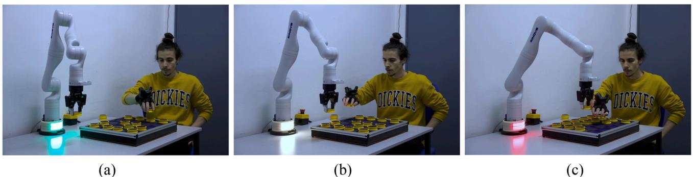
Fig. 6. Collaboration risks. (a) Low risk - green light: there is not any potential detected collision. (b) Medium risk - orange light: the robot has detected a possible collision. (c) High risk - red light: the detected collision is imminent.
