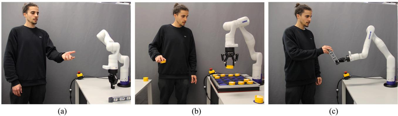
**Fig. 1.** Examples of collaborative tasks in which the human and the robot continuously share both the workspace and the execution of the task. (a) Example of a collaboration in which the human is stopped asking the robot for a tool. (b) Example of a kitting task in which the human and the robot collaboratively fill a tray with tokens. This task was used during the validation. (c) Example of a collaborative hand-over of a tool in which the robot and the human exchange forces.
