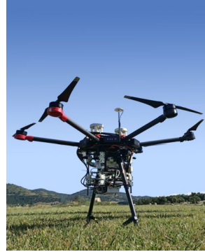
Fig. 9. In the context of the EU H2020 project GAUSS, we equipped a UAV with two GNSS receivers and an IMU. Plain GNSS fixes show numerous multi-path artifacts yielding an erratic trajectory (gray). We combined IMU, GNSS pseudoranges (magenta) and TDCP (cyan) together with robust outlier rejection to achieve smooth and accurate motion estimation (red).
