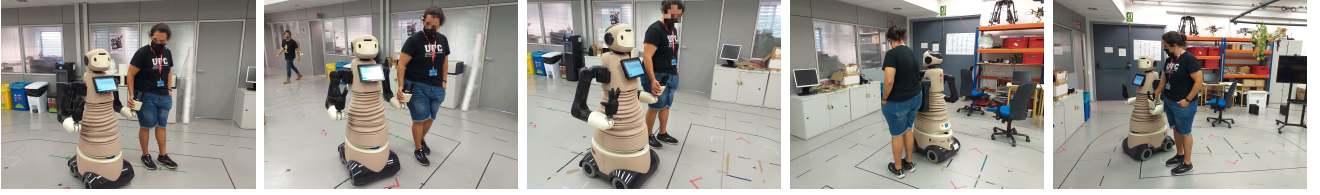
Fig. 3. Guiding the robot task: Sequence of movements turning the robot using physical contact. The robot is controlled using only the F/T sensor.
