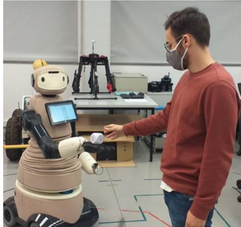
Fig. 1. We use the IVO robot to study how the human motion prediction can help during the hand-over collaborative task.
