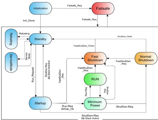
Figure 1. Overall scheme of state machine
