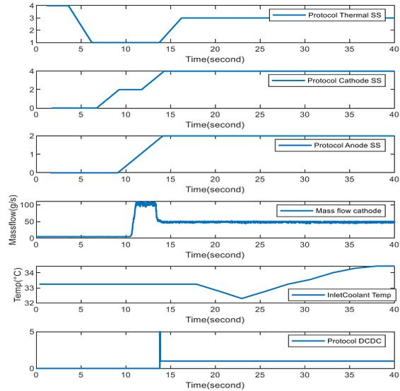
Figure 3. Activation of the subsystems in the startup procedure
