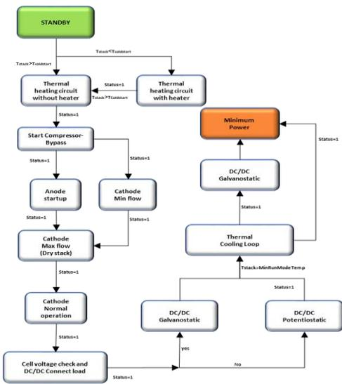
Figure 2. Startup procedure
