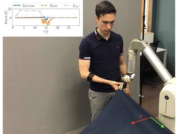
Fig. 1. The main human-robot interaction phase involved in our learning algorithm. The robot follows a reference subject to a perturbing force in  $x$  (the grey curve in the plot), while the human corrects its trajectory if the task specification is violated. The force measurements along the perturbation's axis, obtained with a force sensor and with an electromyography bracelet, are shown in blue resp. orange in the plot.
