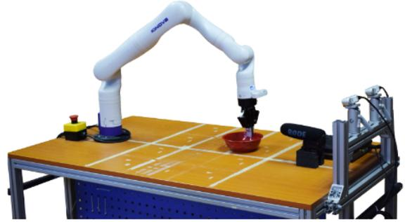
Fig. 1: Experimental setup. Robot manipulator pokes objects with a closed gripper, generating impact sounds used for material classification.
