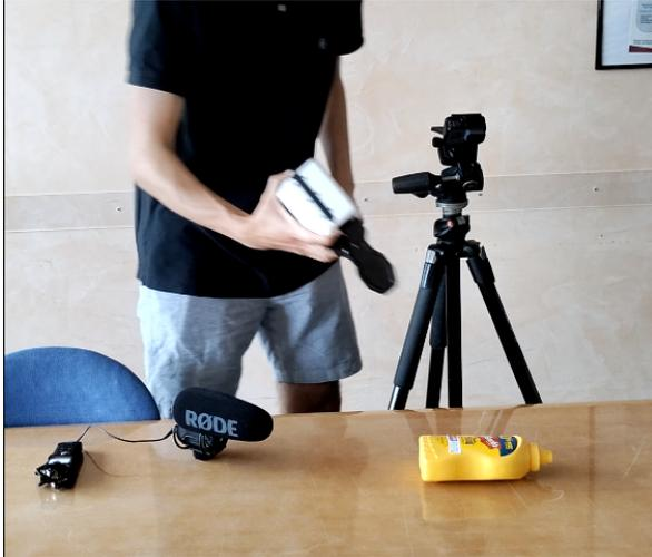
Fig. 2: Capture setup used for our manually collected YCB-impact sounds dataset. A metallic gripper (hold by one hand) is used to interact with the object. Impact sounds generated by the interaction are captured by a shotgun microphone. A static camera is used to capture a close view of the object.
