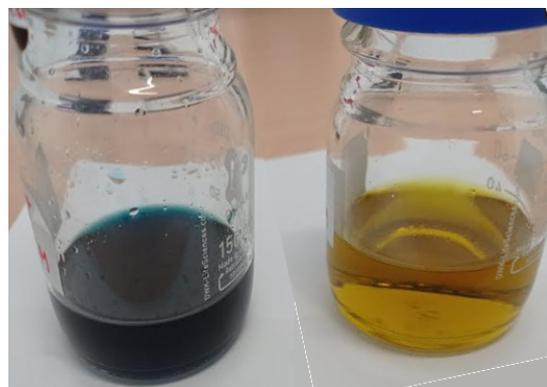
Figure 10: Reservoirs with the original  $V^{3.5+}$  electrolyte (left) and the  $V^{5+}$  concentration electrolyte (right).
