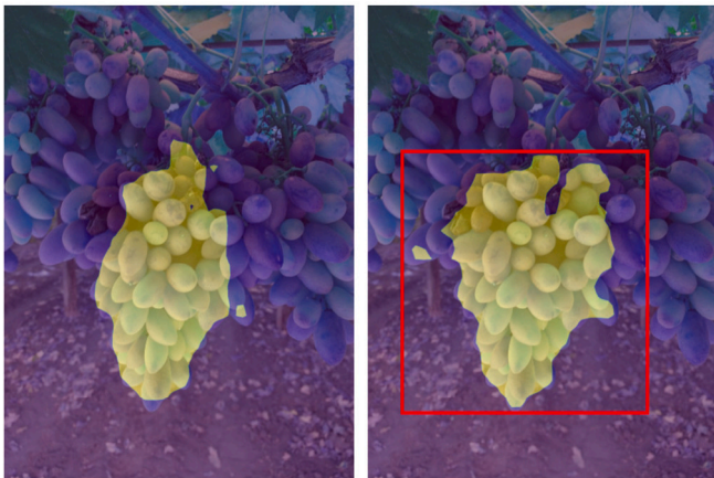
Fig. 10. Left image: pseudo mask produced by Mask-RCNN trained only on the Source Dataset and without a bounding box cue. Right image: same image showing the effect of giving a bounding box cue at inference time.
