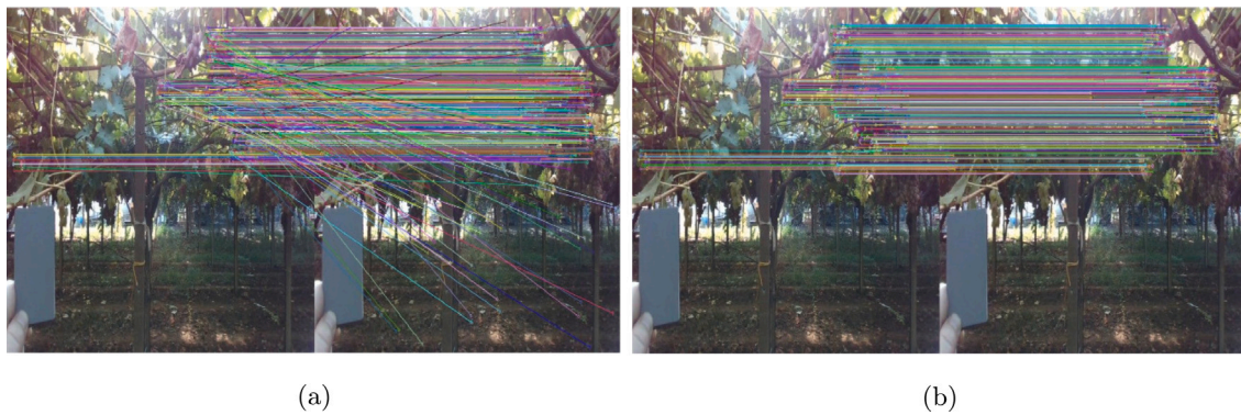
Fig. 6. Feature matching and geometric verification using RANSAC: COLMAP SfM in its lightest form still requires considerable computational time and it is viable only for offline elaborations, while 2D feature matching requires much less computation and potentially runs in real time. (a) The matching of surf features with brute force matching (b) the same matching refined with homography computation combined with RANSAC selection.
