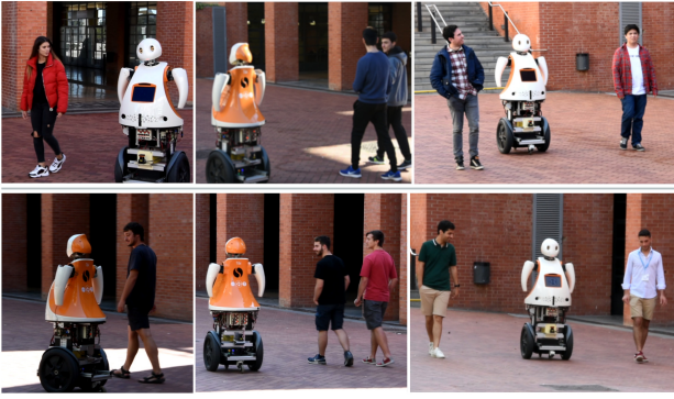
Fig. 1 Real-life Experiments. Top: Three group formations using the ASP-VG method. Bottom: Three group formations using the ASP-SG method. Left: One volunteer is accompanied by our robot, named Tibi, using a Side-by-Side accompaniment. Center: Two volunteers are accompanied by Tibi positioned at the side of each formation. Right: Two volunteers are accompanied by Tibi positioned in the center of each formation.
