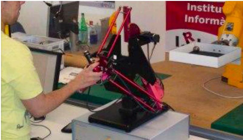
The teacher feels the forces and torques sensed by the force/torque sensor at the robot’s wrist while teleoperating the manipulator with the Delta Haptic Display.
