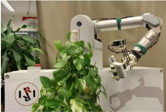
For the GARNICS project, a WAM robot arm holds a time-of-flight camera and two tools for chlorophyll measurement and leaf sample cutting.
