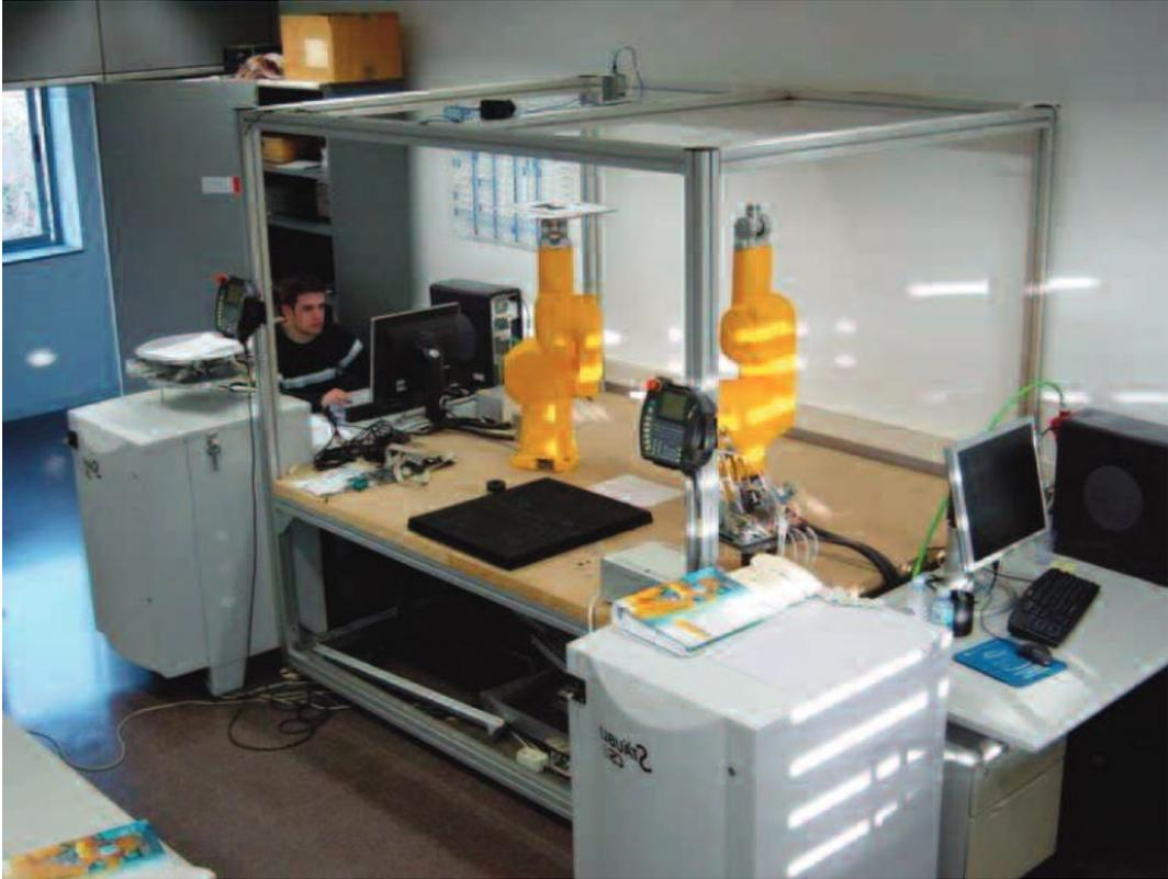
Robotic cell with the two Staubli manipulators.
