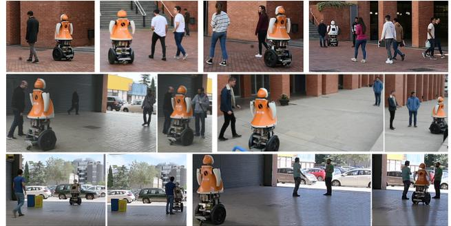
Fig. 1: Different types of HRCN tasks where authors have tested the objective and subjective metrics presented. *Up-left*: Robot Side-by-Side Accompaniment. *Up-right*: Robot V-Form Accompaniment. *Middle*: Robot Accompaniment Plus Approaching. *Bottom*: Robot Approaching.
