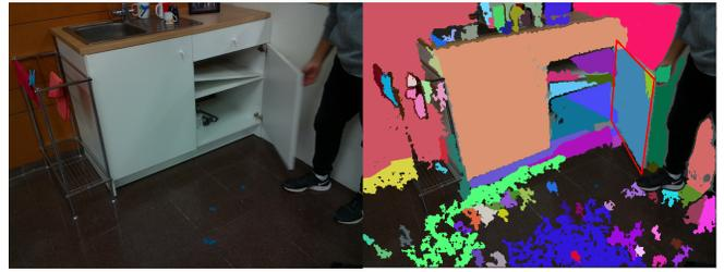
Fig. 3. Input image (left) and a moving part hypothesis denoted by red lines (right). Colored regions in the right image represent detected planar patches.
