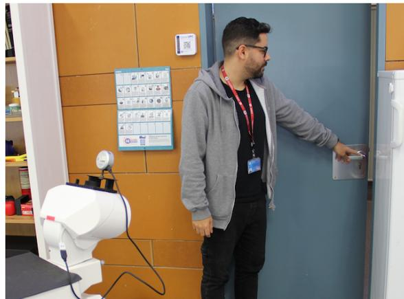
Fig. 1. A human demonstrates to a robot the movement of a door. The robot learns where the door is located and which is the direction of movement.
