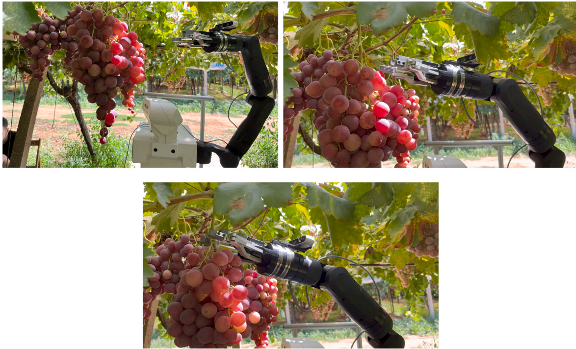
Fig. 3. CANOPIES robot in the field. Top-left: Robot arm with camera in the wrist; Top-right: Cutting tool gripper with stereo camera approaching a grape; Bottom: Cutting tool gripper touching the peduncle.
