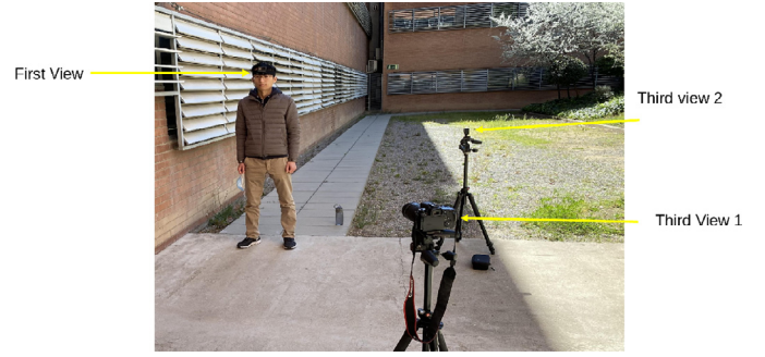
Fig. 2. Capture setup used for our First2Third-Pose dataset. In addition to a head-mounted wearable camera, two static cameras are used to capture side and front views.
