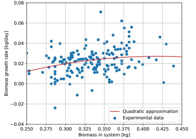
Fig. 2. Experimental data collected at VAXA Technologies Ltd. characterizing the daily biomass growth rate as a function of the biomass available in the culture (the data has been scaled for privacy preserving reasons). The quadratic approximation fit is given in (2).
