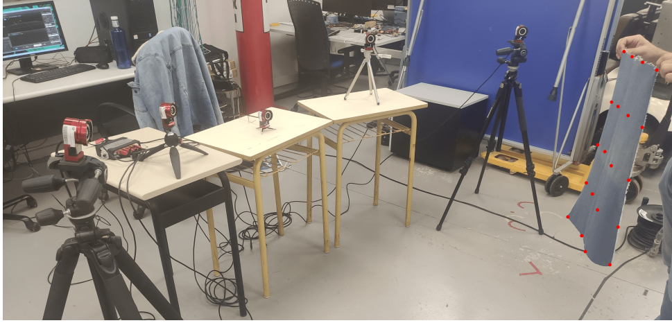
Figure A.11: Setup used to record the motion of the textiles: 5 cameras surround the scene so that every marker (highlighted in red in the photo) is visible to at least 2 cameras at the same time. This ensures that the system can be certain of the 3D position of the marker.
