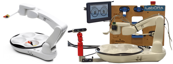
Figure 2: Original Obi device (left) and robotised version (right) able to perform tool change (not used in this work), including RGB-D camera, screen and security button.
