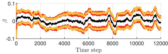
Fig. 5. Set-membership estimation of  $\beta$  using proposed approach (red) and reference approach (orange).
