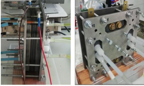
Figure 9: VRFB single cell assembled in the Instituto de Carboquímica center.
