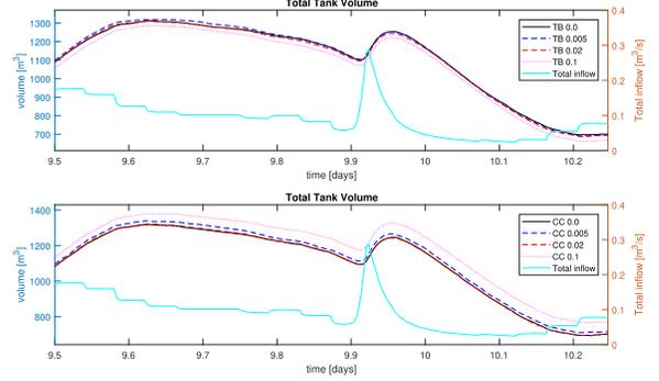
Fig. 5. Tank volumes of T-MPC and CC-MPC with different offsets.
