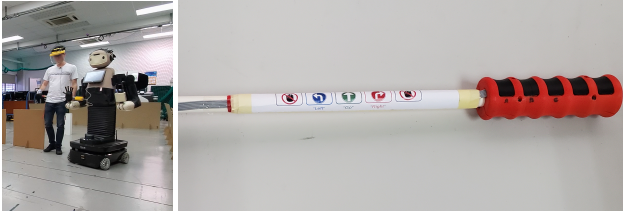
Figure 4: Use case for acceptability study. Left: Human and robot collaboratively transport an aluminium bar through a maze. Right: Transported bar with buttons in the handle and meaning of each button annotated next to it.
