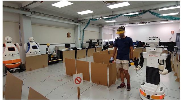
**Fig. 1** Example of Human–robot pair collaboratively transporting an object. Both agents must navigate through a complex environment with multiple walls. Human has extra information since he is the only one to understand the forbidden pass sign. The transported object is a steel bar
