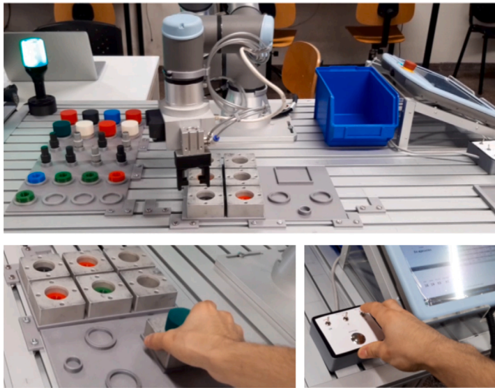
Fig. 6. Quality control scenario. Assembly task of body, bearing, shaft, and cover, with human intervention asking for a quality check.
