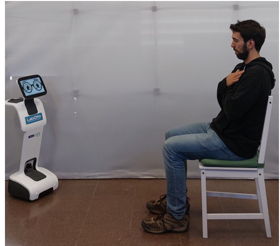
Fig. 1. Showcase of the frailty assessment. The robot monitors the patient (one of the authors) while he starts performing the TUG test.
