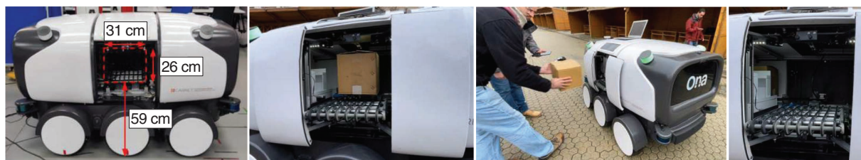
FIGURE 4. Ona's storage management system with four internal compartments.
