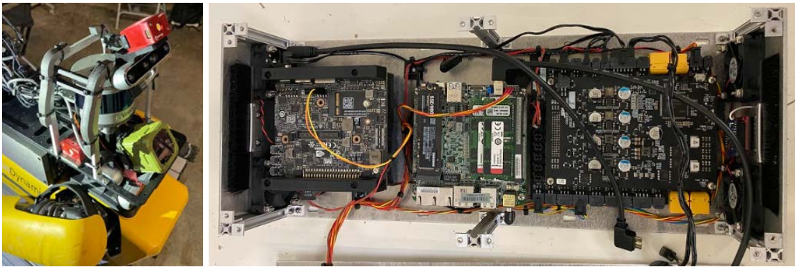
Figure 33: Left to Right: NeBula Sensor Package, and NeBula Computing Core and Diagnostics Board
