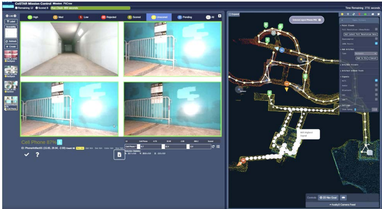
Figure 53: Live operation view during Preliminary Run. Left: The images taken around the area where strong WiFi signals are observed (a clue for Cell Phone artifacts). Right: Pointcloud/topological map built by the robot team with signal strength overlaid.
