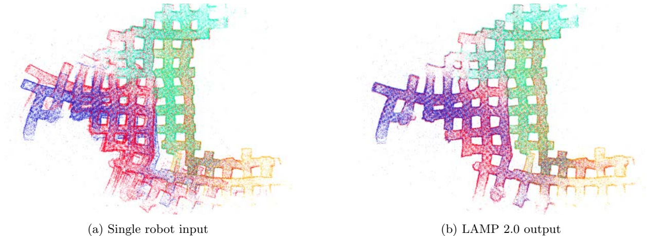
Figure 14: Single-robot map (no loop closures) compared with LAMP 2.0 map (with inter- and intra- robot loop closures) in the Kentucky Underground.
