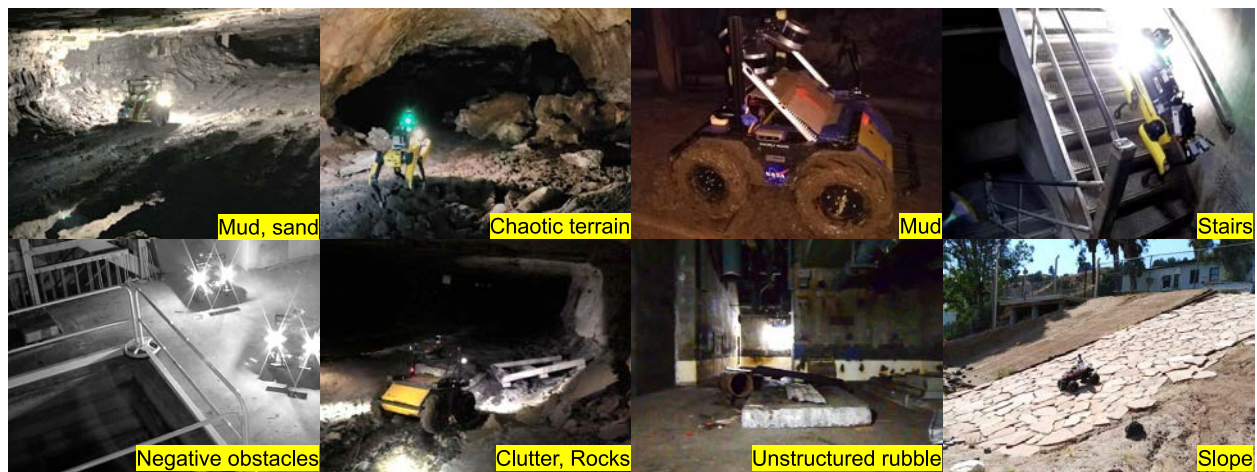
Figure 19: Mobility-stressing elements commonly found during testing in various tunnel, urban, and cave environments, including 800ft underground at Arch Mine in Beckley, WV, Valentine Cave at Lava Beds National Monument, CA, Satsop power plant in Elma, WA, and Mars Yard at JPL, Pasadena, CA.
