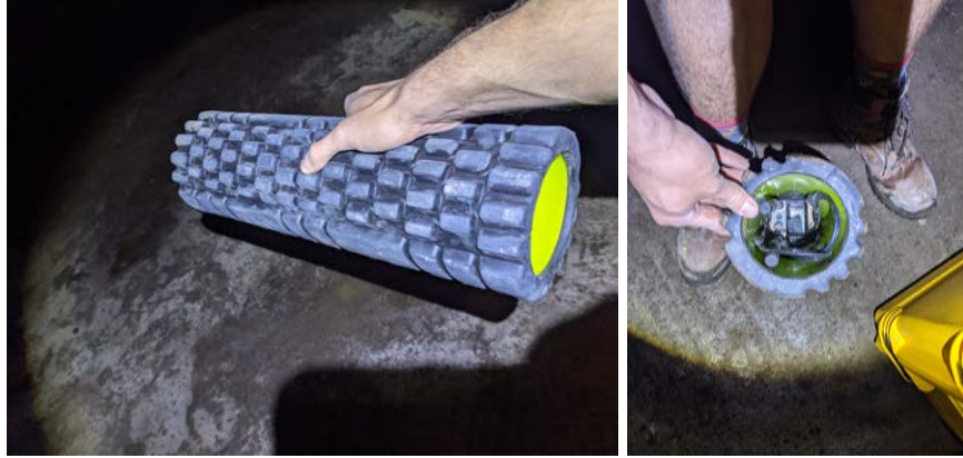
Figure 36: A hand-deployed mesh communication node, a communication roller . The node shown above consists of a Silvus mesh radio and battery fit snugly inside an off-the-shelf athletic foam roller. Although simple, this design reliably protected the radio inside. The communication roller could be deployed from the staging area by rolling the device with a motion similar to throwing a bowling ball. Versions of this communication roller were developed for both aerial and ground robots and were deployed during competition rounds.
