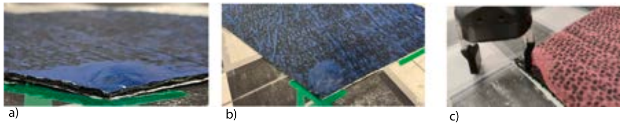
Fig. 14. a) Successful Step 1: the corner sides are completely detached b) Unsuccessful Step 1: the corner sides are still attached to the prepreg c) Most common unsuccessful condition of Step 2.
