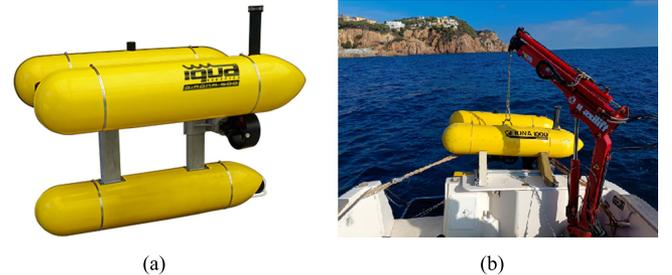
Fig. 2. Girona 1000 AUV from IQUA Robotics. (a) General view and (b) robot deployment at sea using the Sextant boat from Universitat de Girona.
