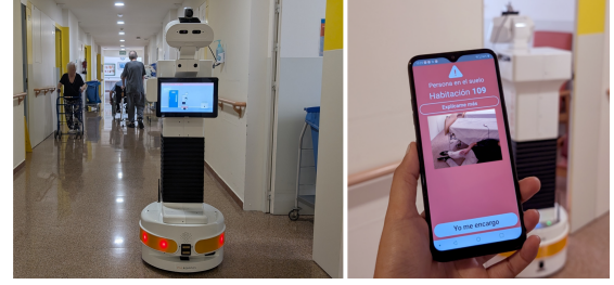
Fig. 2. The robot autonomously returns to its charging station after completing a patrol round (left) and user interface displaying a fall alert actioned from the robot sensors (right).
