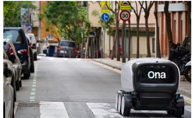
FIGURE 1. ONA, the robot used in our experiments.
