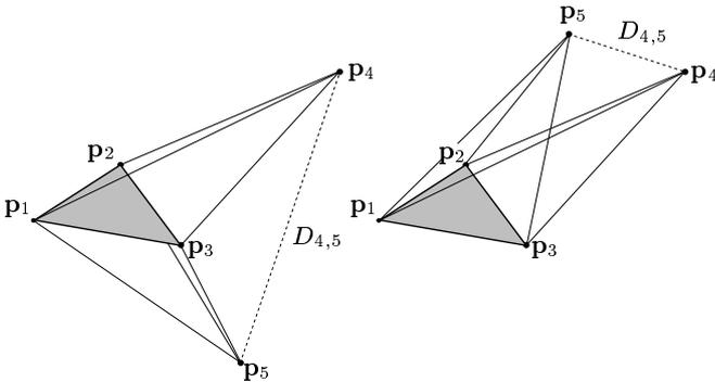
Fig. 2. Computing the location of  $\mathbf{p}_4$  and  $\mathbf{p}_5$  from their distances to  $\mathbf{p}_1$ ,  $\mathbf{p}_2$ , and  $\mathbf{p}_3$  by applying two trilaterations permits finding  $\|\mathbf{p}_5 - \mathbf{p}_4\|$ . Two solutions are possible that depend on the relative location of  $\mathbf{p}_4$  and  $\mathbf{p}_5$  with respect to the plane defined by points  $\mathbf{p}_1$ ,  $\mathbf{p}_2$ , and  $\mathbf{p}_3$ .
