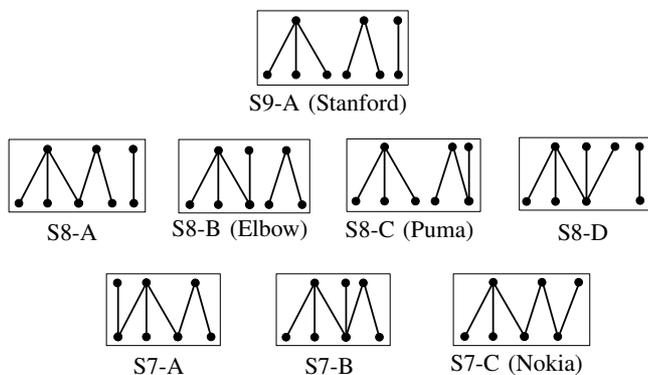
Fig. 6. Schematic representation of all trilaterable serial robots.
