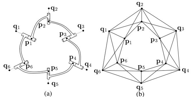
Fig. 5. A general 6R mechanism (a), and its representation in terms of distance constraints (b).
