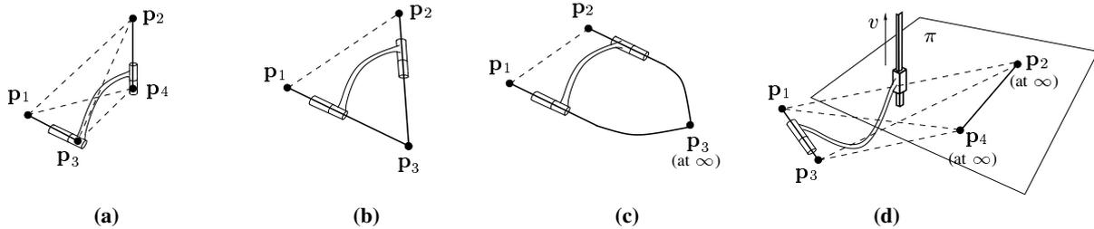
Fig. 1. Modelling a link as a set of points with some fixed distances between them.
