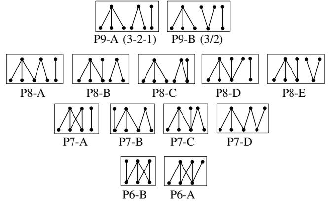
Fig. 4. Schematic representation of all trilaterable in-parallel robots.
