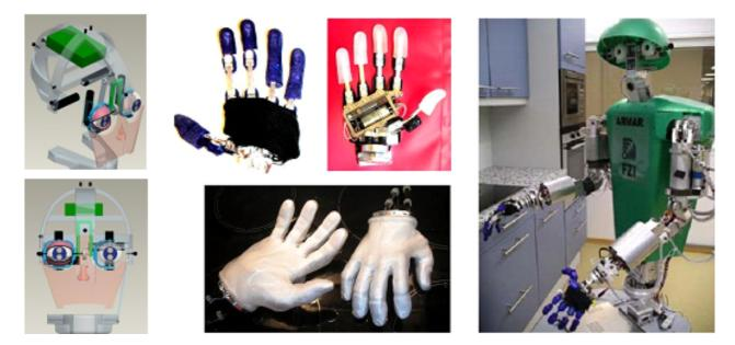
Fig. 1. Model of the proposed new robot head with two cameras for each eye (left), prototype of the five-finger FZK-hand (middle) and the humanoid robot ARMAR (right), Universität Karlsruhe.
