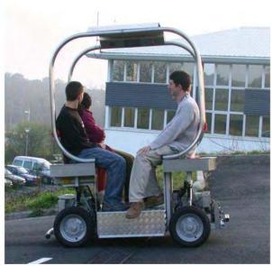
Fig. 9. Robucab mobile robot platform transporting four people.
