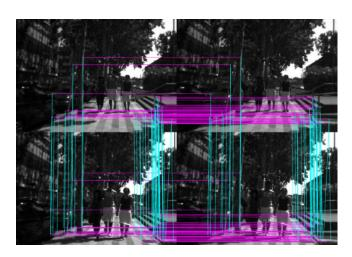
Fig. 1. SIFT correspondences in two consecutive stereo image pairs after outlier removal using RANSAC.
