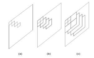
Figure 3: Distribution of features: (a) 4x4 square-blocks: each block is calculated directly form the gradient image and they are not overlapping (b) 8x8 square-blocks: each block is calculated from 4 blocks of the previous level and they are overlapping each other of 50% (c) 16x16 square-blocks: each block can be calculated either with 16 blocks of size 4x4 or with 4 of size 8x8. They are overlapping each other of 75%.
