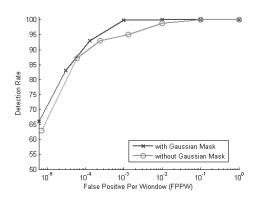
Figure 4: ROC curve of two detectors with different HOG features.
