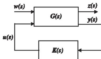
Fig. 8. A sketch of a generic closed loop control system.
