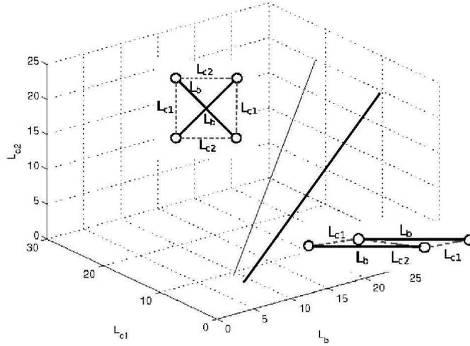
Fig. 5. Two feasible regions for Snelson's X. The thick line is the feasible region for the complete structure and the thin line is the feasible region when the upper cable  $L_{c2}$  is removed. The corresponding configuration is depicted next to its feasible region.
