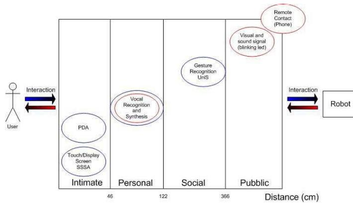
Fig.2: Interaction between the user and the robot across different distances
