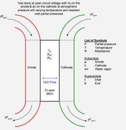
Fig. 1. Schematic diagram of fuel cell water transport model
