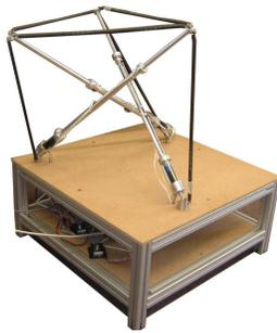
Fig. 8. Tensegrity based prototype robot.
