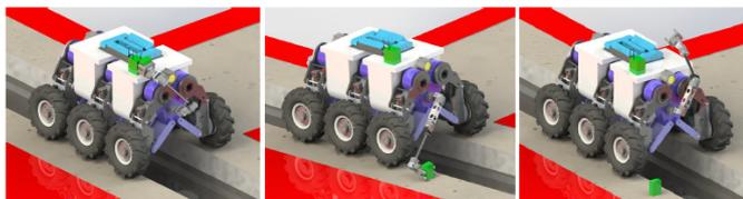
Fig. 3. SIAR Robot deploying one wifi communication repeater.
