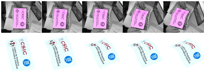
Fig. 13. Paper bending sequence. Top: Images #20, #40, #60, #80 and #100 of a piece of paper under bending deformations with reconstructed mesh. Notice how the 3D mesh is correctly projected and bent into the image. We also show our automatic re-texturing of the paper sequence that is sequentially executed. Bottom: General view of the textured 3D reconstruction seen from a different viewpoint. Best viewed in color.
