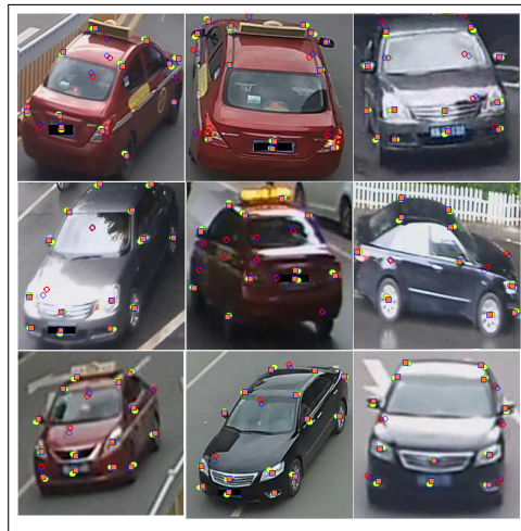
Fig. 5. Results of keypoint detection vs. ground truth labeling considering also self-occluded points in the vehicle. The yellow circles are the predictions and the red squares mark the ground-truth with non-occluded points. Blue circles are ground truth, and red circles are predictions of keypoint position with self-occluded points (partially or totally occluded).
