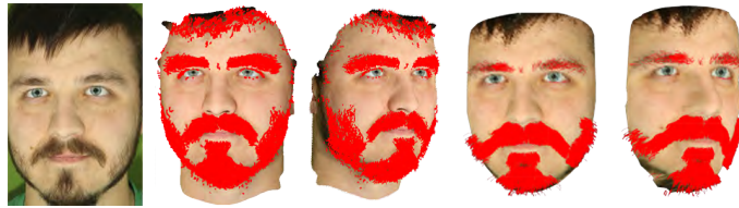
Fig. 6. Qualitative comparison on 3D hair+face reconstruction. First column: input RGB image for our approach. It is worth noting that the solution in [4] requires 14 cameras along with 4 flashes, i.e., a very constrained calibration is demanded. Second and third column: frontal and side views using [4]. Fourth and fifth column: our solution.
